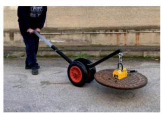
Innovative device for lifting steel and cast iron manhole covers up to 100Kg. All-terrain system with large-diameter, puncture-proof wheels and linear bearings. Sugarlift can be used at different heights, on the construction site, on roads, sidewalks and roads.
