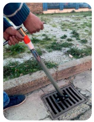
\*Not recommended for use on heavier manhole covers, because the magnet is never in optimal conditions to work at 100% (surface that is not totally flat, irregular drawing of the lid, dirt or dust in the grip area...)
